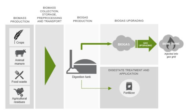
Figure 3. Production pathway for biomethane produced through anaerobic digestion
